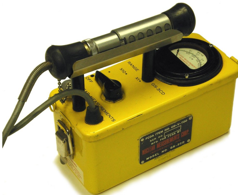
Figure 6.44 Practical GM tube with measuring device
